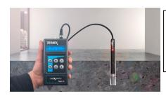
In Situ testing measures the conditions of the concrete slab at a depth of 40% of the overall thickness and gives invaluable evidence needed to ensure a good install and long lasting performance of the flooring material.
